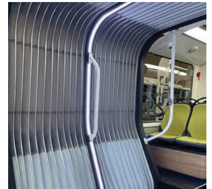
The new Ecoflex bellows with integrated lighting.
